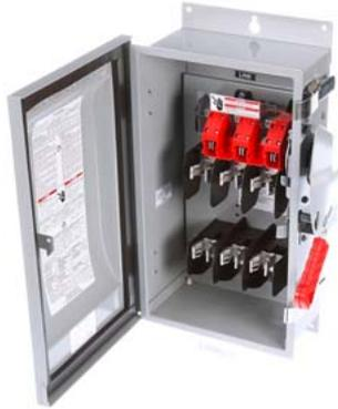
Siemens Low Voltage Circuit Protection Heavy Duty Safety Switches. Type: ENCLOSED, SAFETY SWITCH Std: UL V. Rating: 240V A. Rating: 30 A Wattage: 3W No. Of Poles: 3P F. Rating: 60Hz Action: SINGLE THROW Material: 304SS Enclosure: TYPE 12. 2-3 point mounting holes. Insulation: YES O. Cycles: 10000 O. Temperature: (-20F-120F) AMBIENT TEMPERATURE Environmental Conditions: INDUSTRIAL
