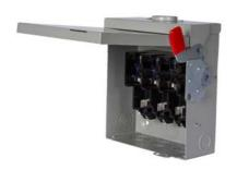
Siemens Low Voltage Circuit Protection General Duty Safety Switches. Type: ENCLOSED, SAFETY SWITCH Std: CSA V. Rating: 240V A. Rating: 200A Wattage: 3W No. Of Poles: 2P F. Rating: 60Hz Action: SINGLE THROW Material: STEEL Enclosure: TYPE 1. 2-3 point mounting holes. O. Cycles: 8000 O. Temperature: (-20F-120F) AMBIENT TEMPERATURE Environmental Conditions: INDOOR
