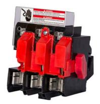
Siemens Low Voltage Circuit Protection Heavy Duty Safety Switches. Type: ENCLOSED, SAFETY SWITCH Std: UL V. Rating: 240V A. Rating: 30 A Wattage: 3W No. Of Poles: 3P F. Rating: 60Hz Action: DOUBLE THROW Material: 304SS Enclosure: TYPE 3R. 2-3 point mounting holes. O. Cycles: 10000 O. Temperature: (-20F-120F) AMBIENT TEMPERATURE Environmental Conditions: OUTDOOR
