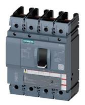
circuit breaker 3VA5 UL frame 250 breaking capacity class H 65kA @ 480V 4-pole, line protection TM210, FTFM, In=90A overload protection Ir=90A fixed short-circuit protection Ii=10 x In N conductor protection 100% without connection
