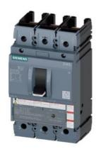
circuit breaker 3VA5 UL frame 250 breaking capacity class M 35kA @ 480V 3-pole, line protection TM210, FTFM, In=250A overload protection Ir=250A fixed short-circuit protection Ii=10 x In UL 489 SB (naval), 50 °C without connection
