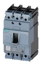
circuit breaker 3VA5 UL frame 125 breaking capacity class S 25kA @ 480 V 3-pole, line protection TM230, FTAM, In=40A overload protection Ir=40A fixed short-circuit protection Ii=5...10 x In UL489 SB (naval), 50 deg. cel. cable connection on both sides
