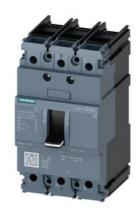
circuit breaker 3VA5 UL frame 125 breaking capacity class S 25kA @ 480 V 3-pole, line protection TM210, FTFM, In=110A overload protection Ir=110A fixed short-circuit protection Ii=10 x In UL489 SB (naval), 50 deg. cel. nut keeper kit on both sides
