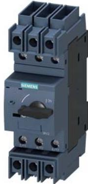
Circuit breaker size S00 for transformer protection with approval circuit breaker UL 489, CSA C22.2 No.5-02 A-release 15 A N-release 286 A screw terminal Standard switching capacity
