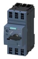
Circuit breaker size S00 for transformer protection A-release 7...10 A N-release 208 A Spring-type terminal Standard switching capacity
