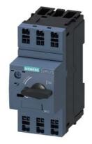
Circuit breaker size S00 for transformer protection A-release 4.5...6.3 A N release 130 A Spring-type terminal Standard switching capacity
