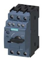
Circuit breaker size S00 for transformer protection A-release 0.18...0.25 A N-release 5.2 A screw terminal Standard switching capacity with transverse auxiliary switches 1 NO+1 NC
