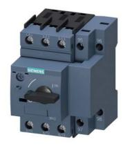
Circuit breaker size S00 for motor protection, CLASS 10 with overload relay function A-release 0.28...0.4 A N-release 5.2 A screw terminal Standard switching capacity
