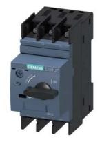
Circuit breaker size S00 for motor protection, CLASS 10 A-release 10...16 A N-release 208 A ring cable lug connection Standard switching capacity
