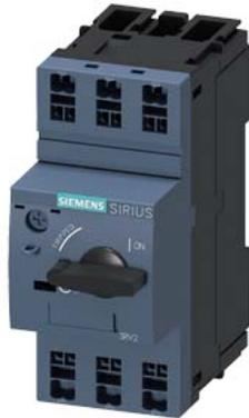
Circuit breaker size S00 for motor protection, CLASS 10 A-release 3.5...5 A N release 65 A Spring-type terminal Standard switching capacity
