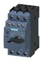
Circuit breaker size S00 for motor protection, CLASS 10 A-release 2.8...4 A N release 52 A screw terminal Standard switching capacity with transverse auxiliary switches 1 NO+1 NC
