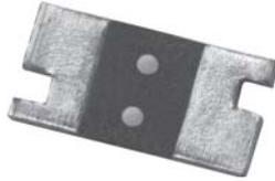
The CSM's series of low value current sense resistors provides power and precision in a four terminal, surface mount configuration. Its all welded construction is made up of a Bulk Metal® resistive element with plated copper terminations.
