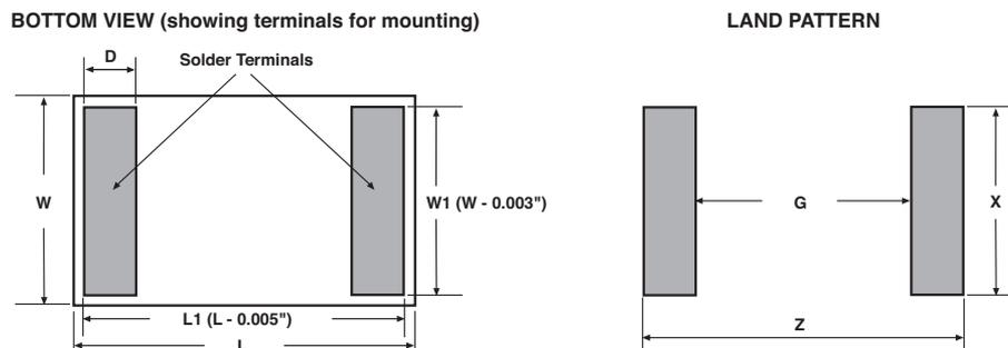
**Note:** Recommended stencil thickness 0.2 mm/0.00787 inch minimum
