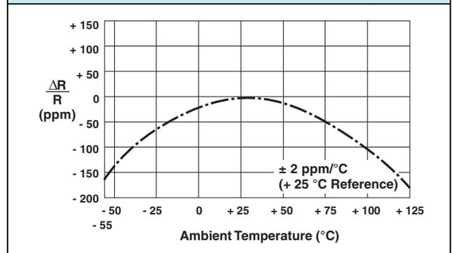
**Note:** The TCR values for < 80 Ω are influenced by the termination composition and the result in deviation from this curve
