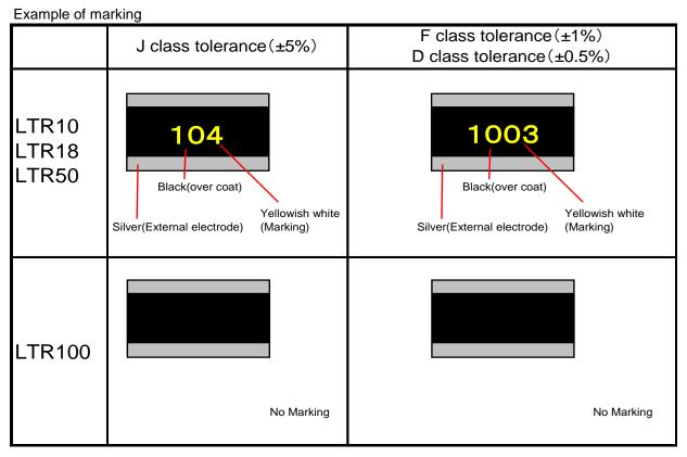
① Marking method : There are three or four digits used for the calculation number according to IEC code and "R"is used for the decimal point.
