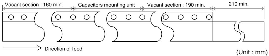
(6) The top tape or cover tape and base tape are not attached at the end of the tape for a minimum of 5 pitches.
