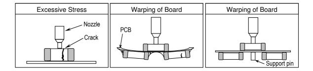
typically adjusted to 1N to 3N (static load) during the pick and place operation.
