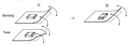
5.2 Crack will be caused if board is warped due to excessive load by check pin.
