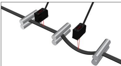
**Electrode thickness measurement**
