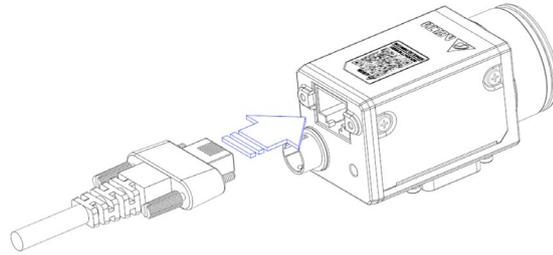
7. Connect the 6-pin GPIO cable. DC power supply or I/O functions should be wired according to the DMV-C I/O definition to ensure normal functioning. If DC power supply or I/O functions are not used, this step can be skipped.
