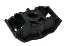
Separates bundles to help prevent chafing and wear. Single bundles can be mounted on top of the mount, or two bundles can be separated using the two side saddles; giving the mount versatility.
