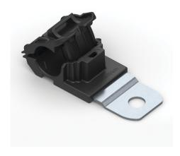
Ratchet P-Clamp, 0.50 - 0.77" Bundle Dia, 180° Short, 0.33" Hole Dia, PA66HIRHSUV/ST/ZN, Black, 20/bg
