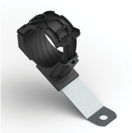
Ratchet P-Clamp, 1.38 - 2.01" Bundle Dia, 30° Long, 0.33" Hole Dia, PA66HIRHSUV/SS304, Black, 140/ctn
