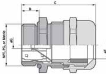
SKINTOP® MS-SC is uniquely designed to address EMI concerns with its simplified grounding feature. In a few easy steps the cable is grounded, strain relieved, and sealed from moisture and dust in accordance with IP68. The cable glands' contact springs establish a continuous electrical path from the shield of the cable to the equipment ground, creating a secure shield connection.
