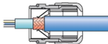
for thin wires without an inner sheath
