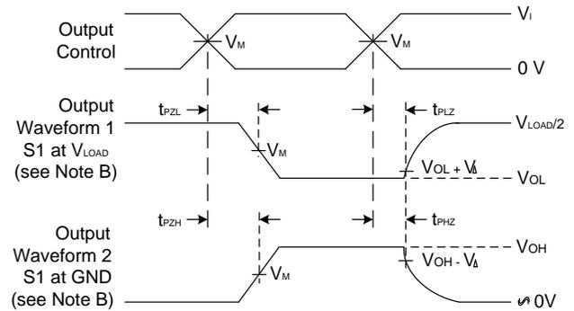
**Figure 1. Load Circuit and Voltage Waveforms**
