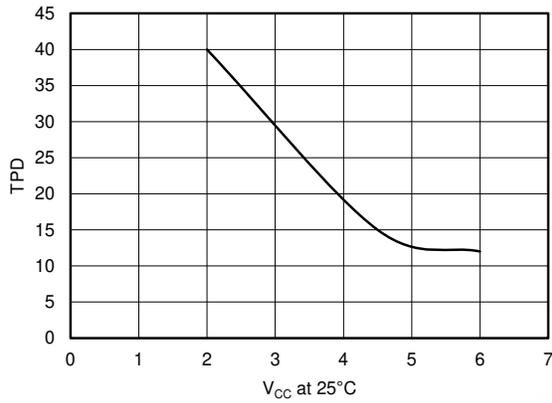
**Figure 5-1. TPD vs V<sub>CC</sub> at 25°C**
