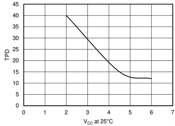
**Figure 5-2. TPD vs V<sub>CC</sub> at 25°C**
