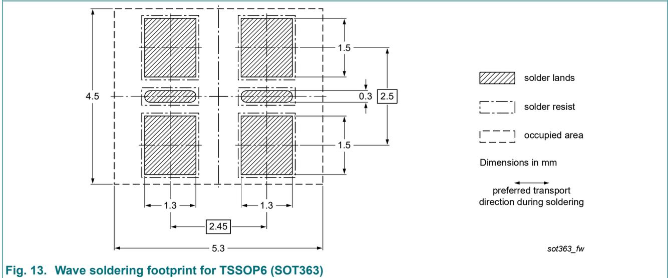
Fig. 13. Wave soldering footprint for TSSOP6 (SOT363)
