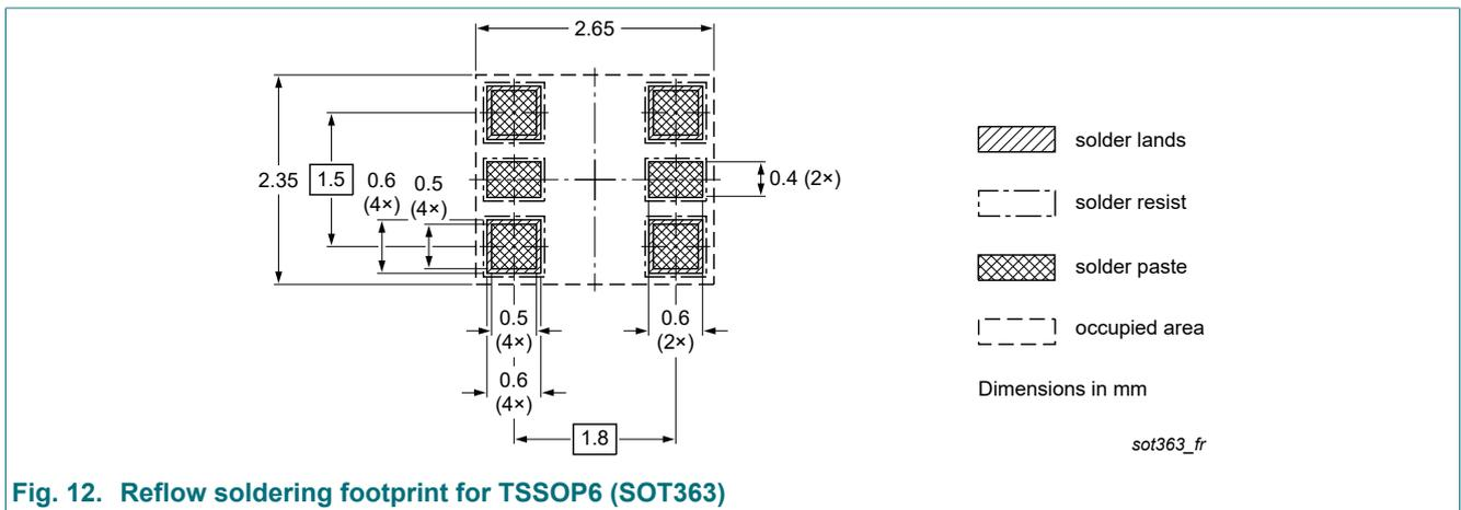
Fig. 12. Reflow soldering footprint for TSSOP6 (SOT363)
