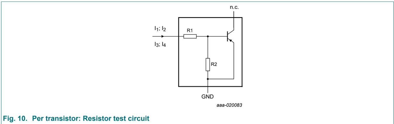
Fig. 10. Per transistor: Resistor test circuit
