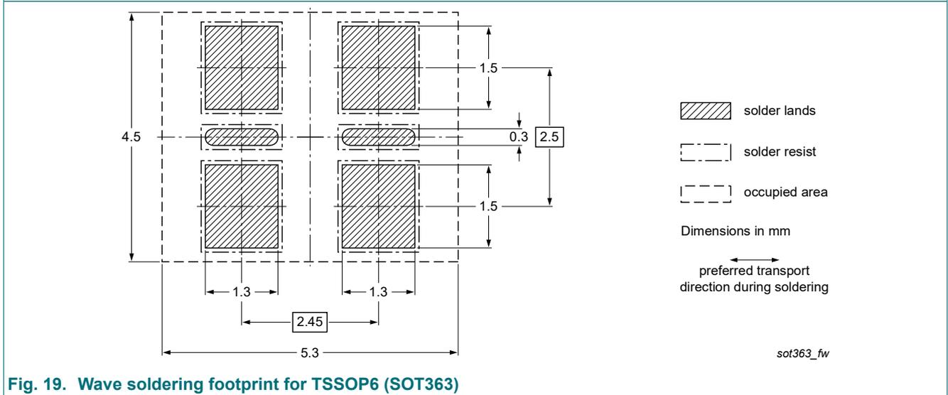
Fig. 19. Wave soldering footprint for TSSOP6 (SOT363)
