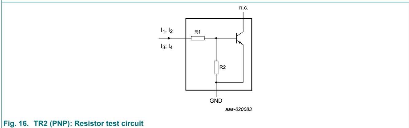
Fig. 16. TR2 (PNP): Resistor test circuit
