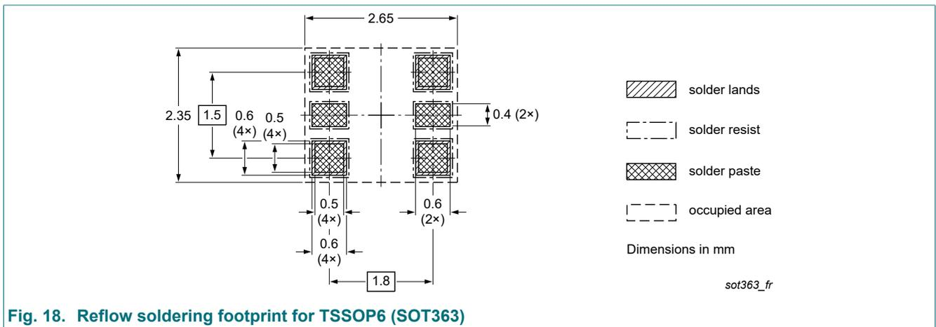
Fig. 18. Reflow soldering footprint for TSSOP6 (SOT363)
