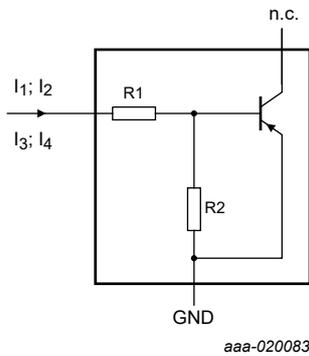
Fig. 7. PNP transistor: Resistor test circuit
