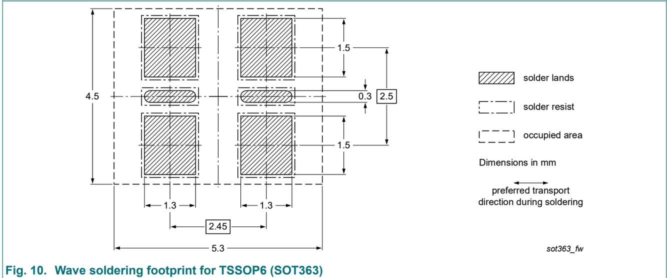
Fig. 10. Wave soldering footprint for TSSOP6 (SOT363)
