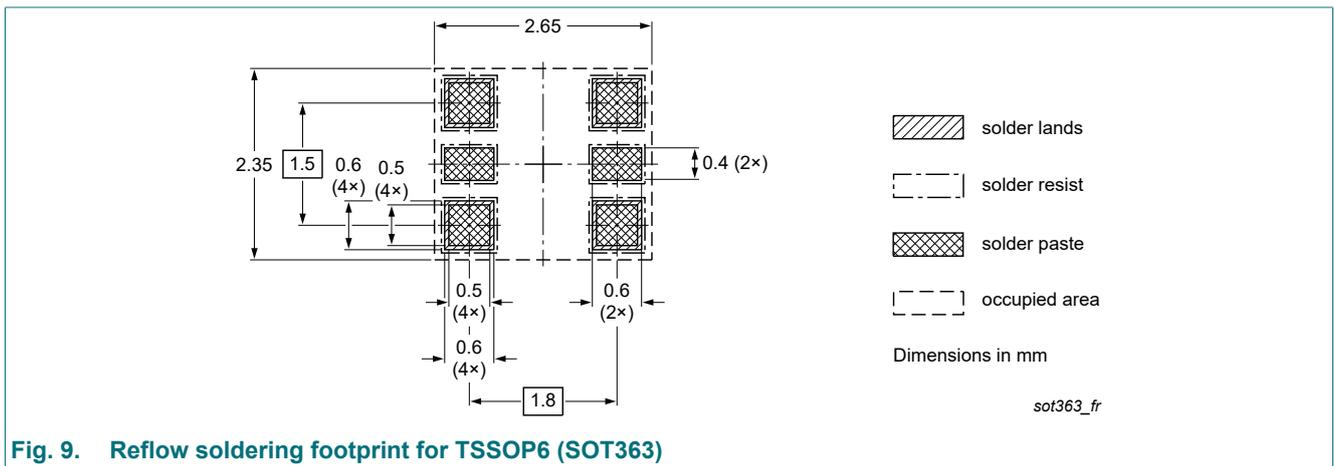
Fig. 9. Reflow soldering footprint for TSSOP6 (SOT363)
