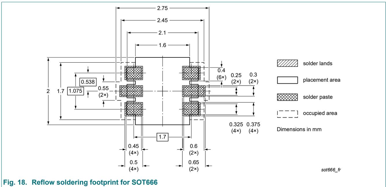
Fig. 18. Reflow soldering footprint for SOT666
