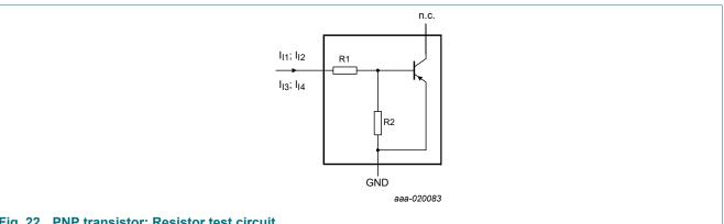
Fig. 22. PNP transistor: Resistor test circuit
