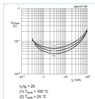
Fig. 19. NHUMB9: Collector-emitter saturation voltage as a function of collector current; typical values
