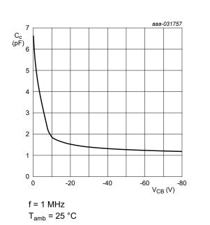
Fig. 20. NHUMB9: Collector capacitance as a function of collector-base voltage; typical values
