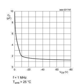
NHUMB10: Collector capacitance as a function Fig. 8. of collector-base voltage; typical values
