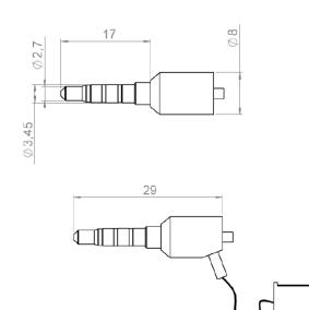
EM059575-0 Audio plug is a highly durable test connector designed for testing 3.5mm audio interface.
