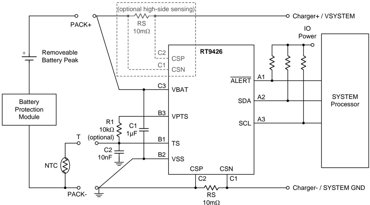
\* Both WL-CSP and WDFN can option High/Low Side NTC
