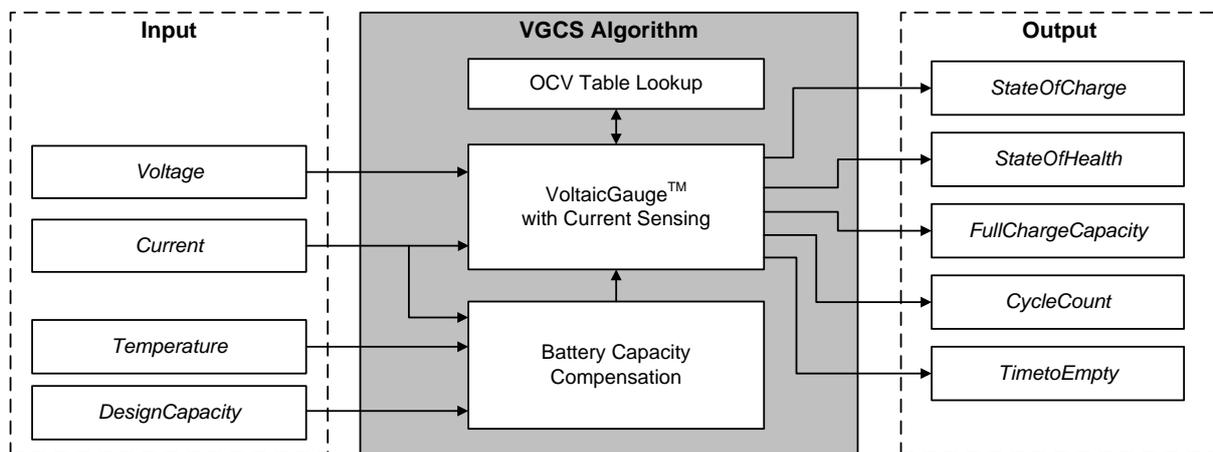
The RT9426 got battery voltage information then using OCV table and iterate calculation with current correction to calculate delta SOC, then using design capacity and battery capacity as a reference to optimize result and output final SOC result. VGCS also support high C-RATE charging technology.
