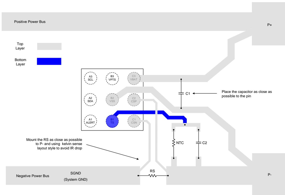
Figure 5. Low-Side Sensing PCB Layout Guide for WL-CSP-9B 2.29x1.74 (BSC) Package
