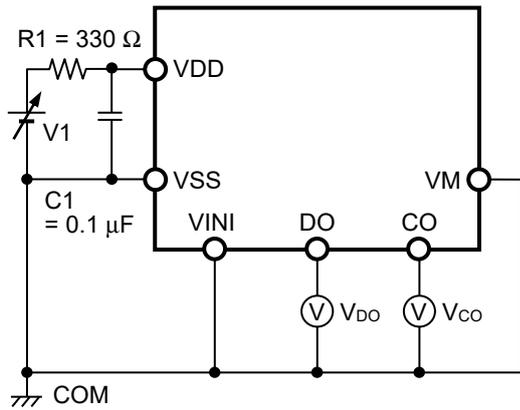
**Figure 3 Test Circuit 1**
