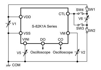
Figure 7 Test Circuit 5
