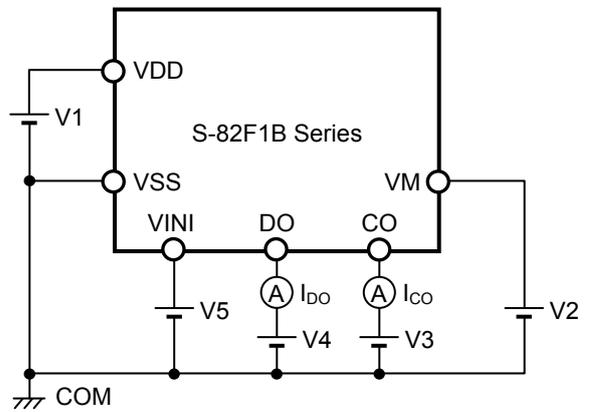
**Figure 6 Test Circuit 4**
