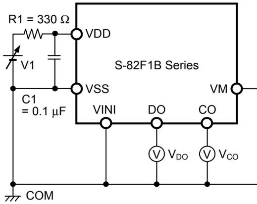
**Figure 3 Test Circuit 1**
