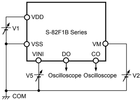
**Figure 7 Test Circuit 5**
