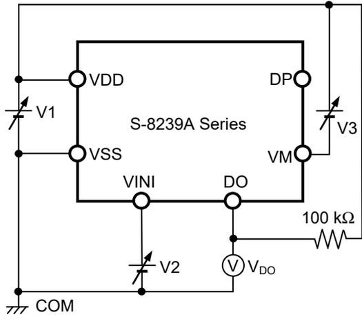
**Figure 4 Test Circuit 1**
