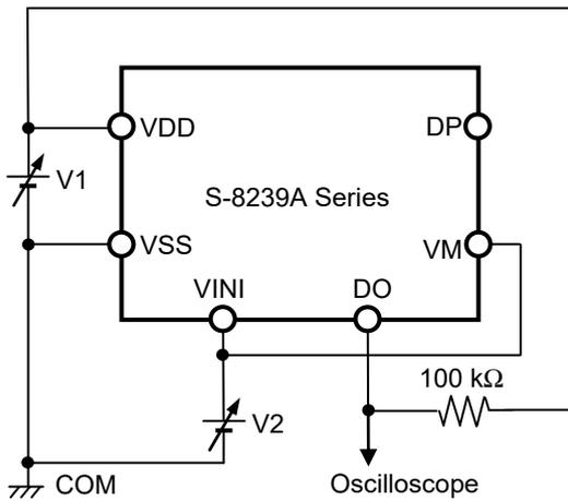
**Figure 8 Test Circuit 5**
