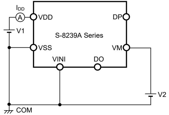
**Figure 5 Test Circuit 2**
