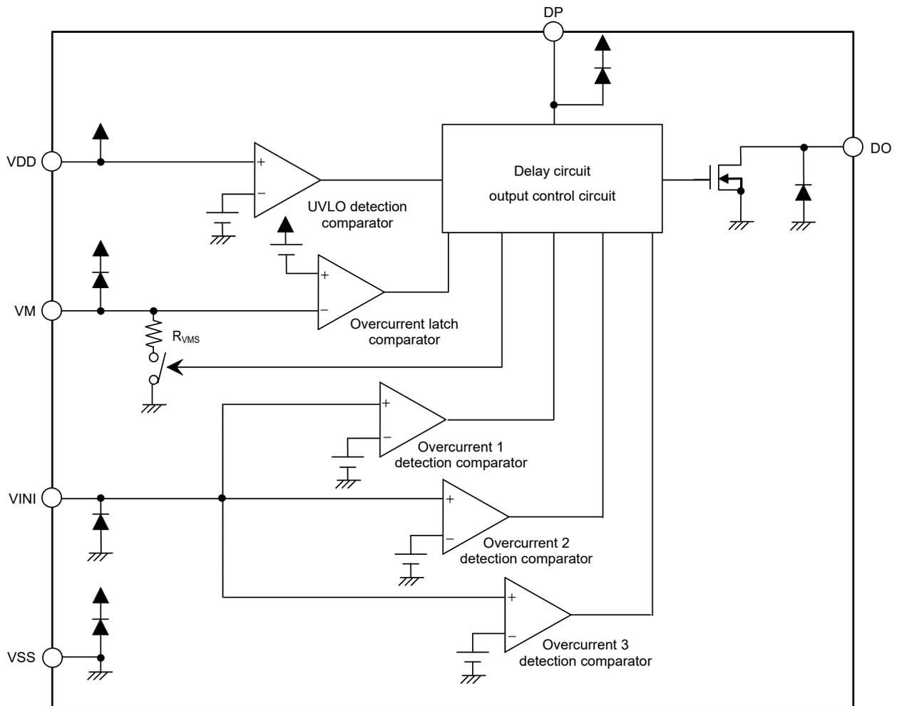
**Remark** All the diodes shown in the figure are parasitic diodes.
