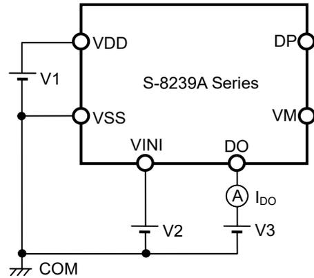
**Figure 7 Test Circuit 4**
