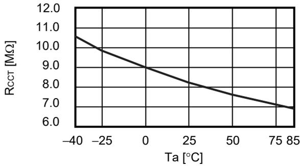
**3.2  $V_{CCT}$  vs  $T_a$  ( $V_{DS} = 18.5 V$ )**
