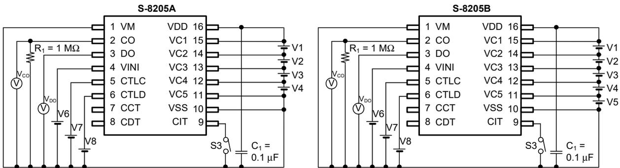
Figure 6 Test Circuit 2
