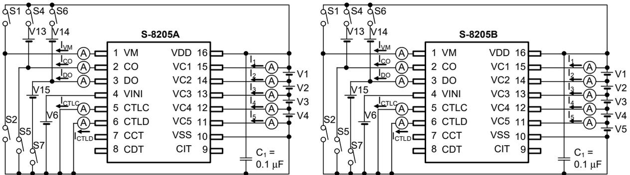
**Figure 9 Test Circuit 5**
