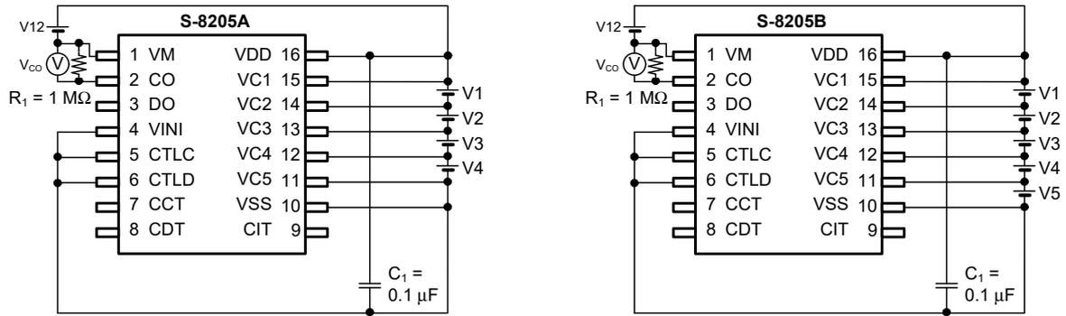
**Figure 8 Test Circuit 4**
