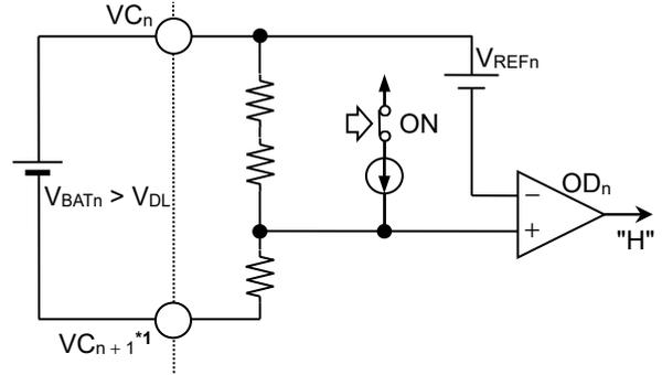
**Figure 21** When Self-test Is Performed (RSTB = "H", CLK = "H<sub>2n</sub>")
