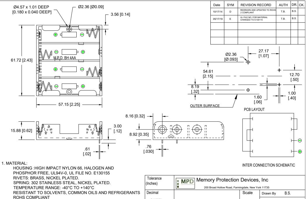
MOUNTING INSTRUCTION: USE 2-56 MACHINE SCREWS OR EYELETS 0.089" OD
