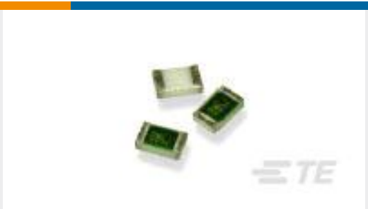
TE Part #2-1614885-7 CPF 0805 910K 0.1% 25PPM 1K RL
