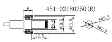
DC PLUG 5.5\*2.0\*12.5mm with 6mm Thumb Screw or equivalent(S761KS12/S761KS15/S761KS17) Mating Switchcraft DC JACK : L722AS/ PCL722AS/L722RAS
