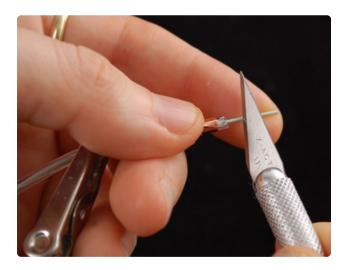
Now that the corona wires are tucked away safely, we can work on soldering to the middle wire. First we must remove the phosphor, by scraping it off. Some people use a lighter to burn it off but we like to just scrape it with a razor. Either way, remove some of it.
