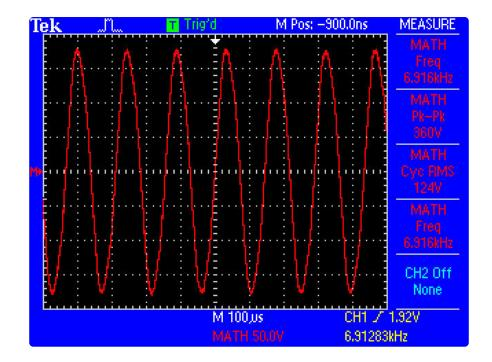
Attaching 3 meters (10 feet) of high brightness EL wire, the frequency stabilizes at 2KHz and 65V, which means we've about maxed out what this driver can provide.
