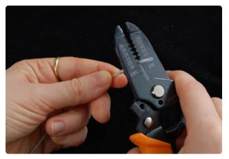
If you arent succeeding at getting the PVC off without damaging the wires, you can try not-quite-closing the cutters all the way (the image below is an exaggeration of how much to close it) and giving it a good yank.
