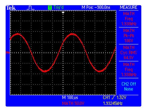
If you are comfortable using tools and want to optimize your driver and wire, you can do so by 'modeling' your EL wire with a capacitor and resistor and plugging that in, then measuring the frequency across the RC with a multimeter or scope, just watch out you don't zap yourself!
