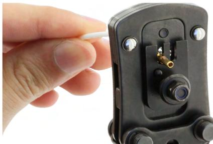
7) Tighten sharply the handles to the end of the mechanism (max 175 N). After handles are opened, extract the contact.
