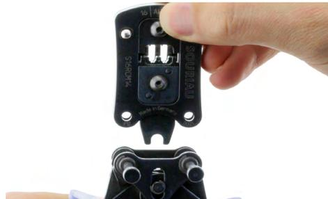
3) Close the two pins simultaneously to maintain the head.
