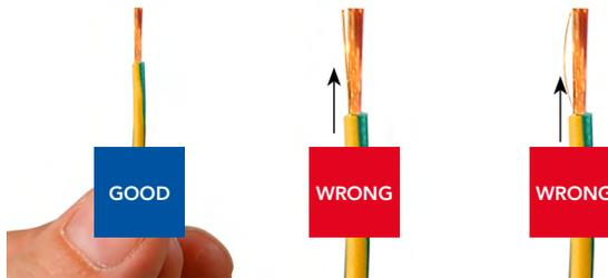
5) Place conductors, with no deterioration, in the contact bucket. All strands to be located in the crimp bucket.
