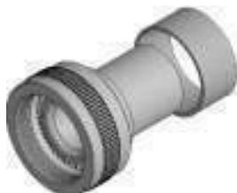
Many cable terminations where heat shrink boots are used will require provision for terminating the screens too. It is achieved in this type of back shell through a ring, which can be crimped to the back shell body holding the screens in between.
