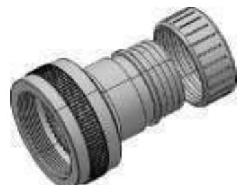
This adaptor is designed with threads similar to that in the lamp base for shield termination. It is very effective, easy and quick method of shield termination and field maintenance is also effortless. The termination area is designed to accept 'Nut' as well as 'Clamp'. The nut option enables the use of heat shrink boot and the clamp option will facilitate the strain relief clamping without heat shrink boot after the shield/cable termination.
