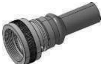
This adaptor is supplied with some length of braid attached. This braid overlaps with the cable braid and effective shielding takes place due to its 360° contact. It is designed to accept heat shrink boot. Ease and less time for cable termination are the prime advantages here.
