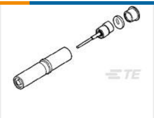
TE Part #222191-1 SOCKET,ARINC,SIZE 8,TRIAxIAL
