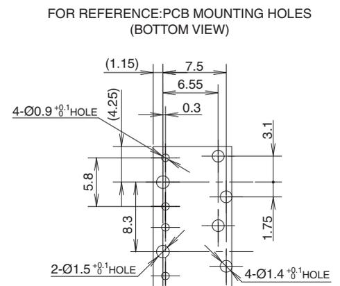
\*Please study & choose other appropriate hole diameters if confirmed the diameter values recommended above don't work with the soldering process.
