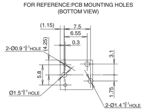
\*Please study & choose other appropriate hole diameters if confirmed the diameter values recommended above don't work with the soldering process.
